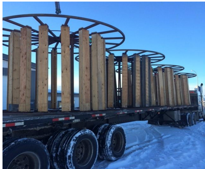
Figure 270: Unacceptable Load of Empty Reels (wooden traverse reels in wrong orientation)
