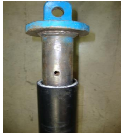
Figure 74: Road Bore Pull Tool
