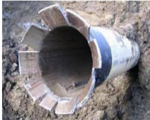
Figure 151: Enlarged Casing Opening
