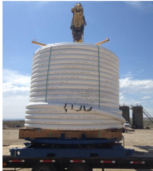
Figure 52: Pipe Coil with Corner Protectors on Pallet
