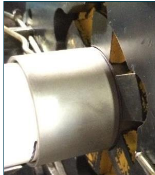
Figure 228: Crimper Dies Aligned with Engraved Crimp Lines
