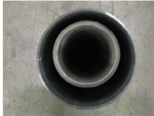
Incorrect positioning of sleeve on mandrel
