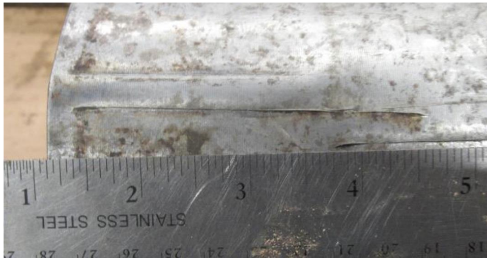
Figure 236: Misaligned 3 rd and 4 th Crimps
