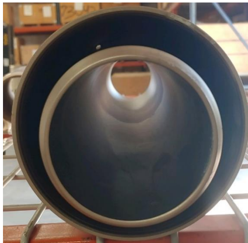
Figure 186: Defect-Free Internal Mandrel Surface
