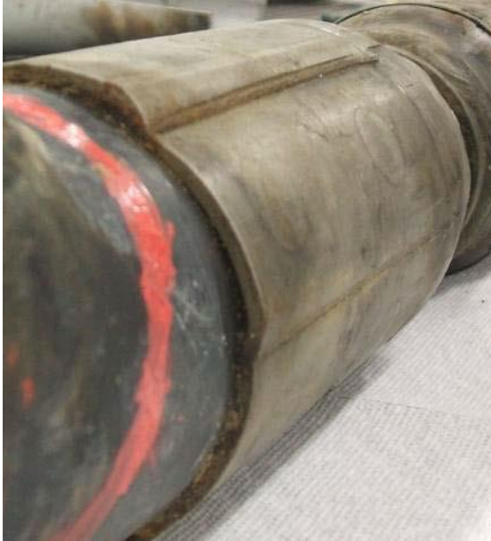
Figure 241: Point Loading on Pipe and No End Flare
