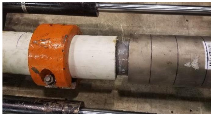
Figure 214: Pipe Clamp Set Closer for Curved Pipe Insertion
