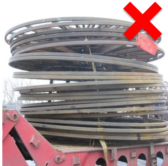
Figure 274: Unacceptable Load of Unassembled Reels
