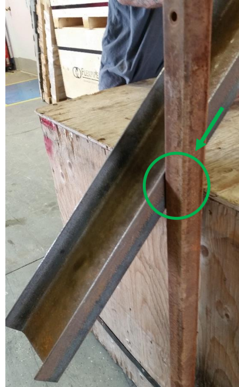
Figure 161: Welding Location for Support
