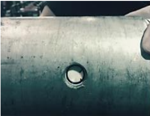
Figure 76: Mark and Drill the Holes
