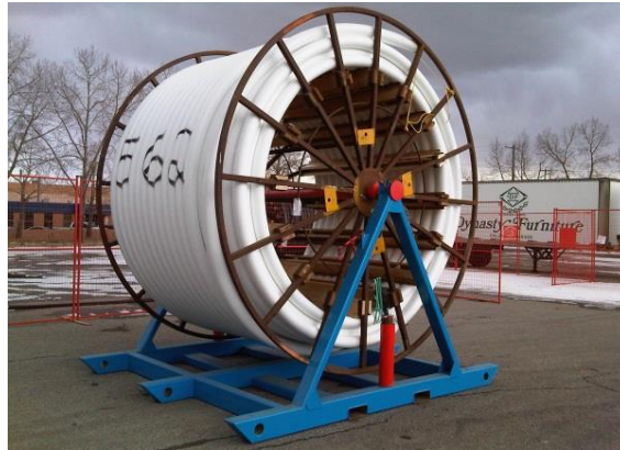
Figure 12: A-Frame Supporting a Reel
