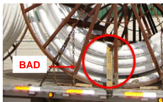
Figure 21: Improper Strapping of Pipe
