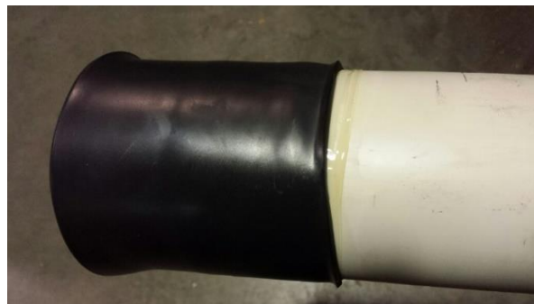
Figure 51: Heat shrink cap installed on a pipe end
