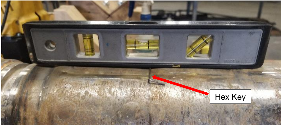
Figure 235: Crimp Gap Checked with Hex Key
