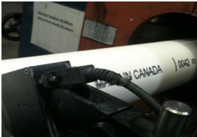
Figure 5: Applying the Print String to Finished Pipe
