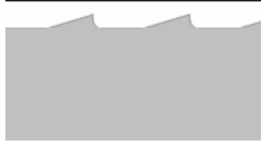
Figure 212: One-Way Teeth on the Pipe Clamp
