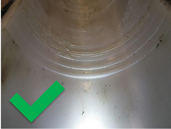
Figure 237: Good O-ring Seal
