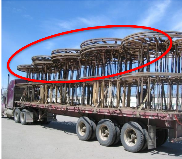
Figure 269: Unacceptable Load of Empty Reels (flanges on top of reels)
