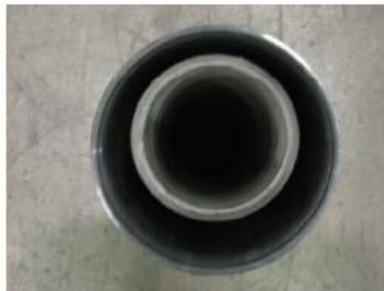
Figure 60: Incorrect Positioning of Sleeve on Mandrel
