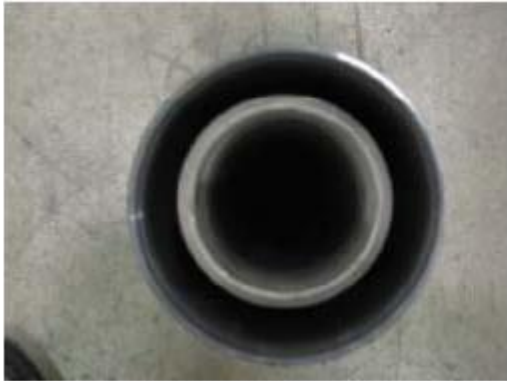
Correct positioning of sleeve on mandrel
