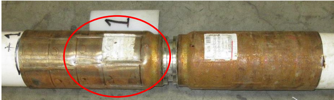
Figure 232: Recessed Crimp Due to Liner Gouge
