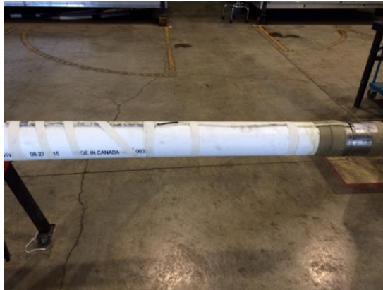
Figure 251: Anode Lead Wire Secured to Pipe
