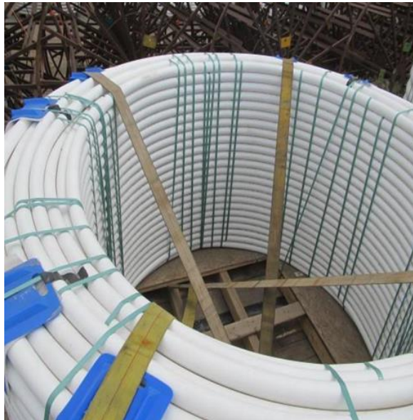
Figure 43: Coil loaded and secured on trailer
