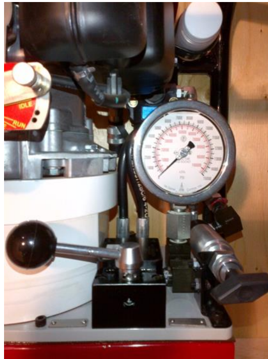
Figure 170: Pressure Gauge on Hydraulic Pump Unit
