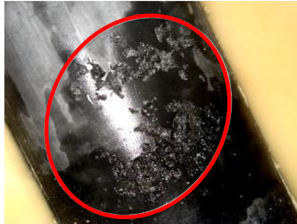
Figure 268: Pitting and Abrasion Hydrovac Damage
