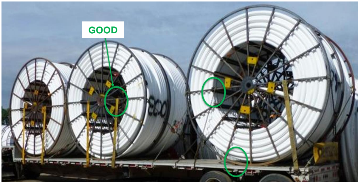
Figure 20: Reels Secured on Trailer
