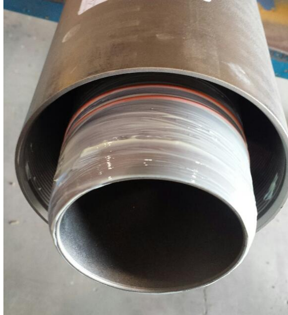
Figure 201: Properly Applied Grease to Mandrel and O-Rings
