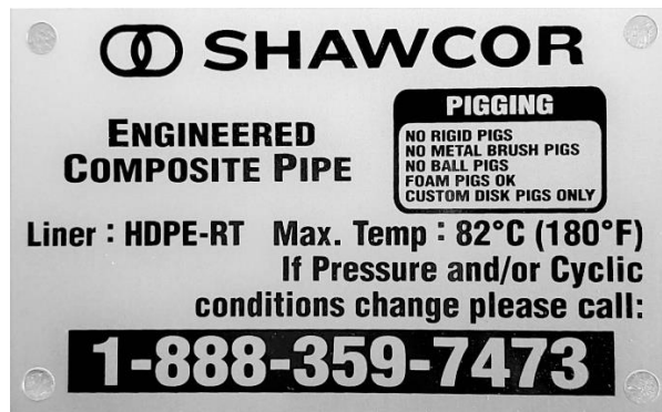
Figure 266: High Temperature Pigging Tag
