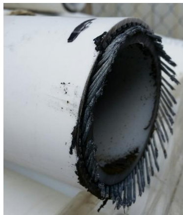
Figure 193: Protruding Cords That Must Be Trimmed
