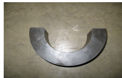
Use Correct Pipe Centering Tool for 2" and 3" Pipe
