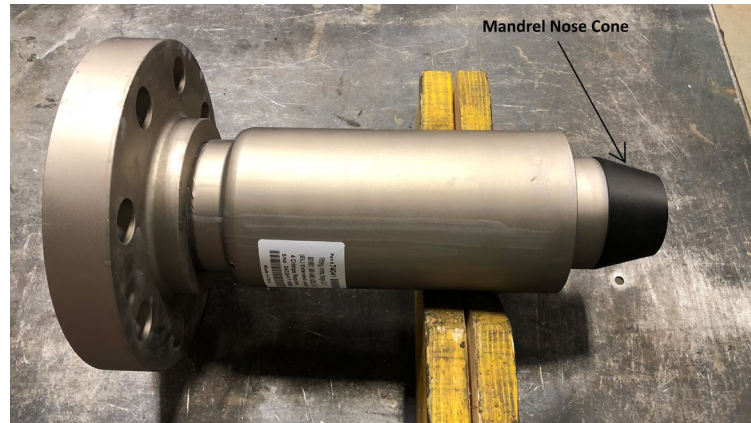
Mandrel Nose Cone Temporarily Attached to a Fitting
