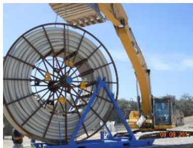
Figure 5: Proper lifting technique, lifting with rated chains or slings attached to the yellow lifting blocks.
