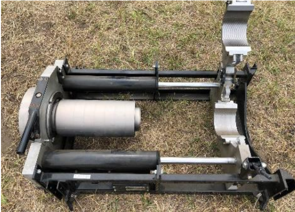
Figure 26: Mandrel Insertion Press on the ground
