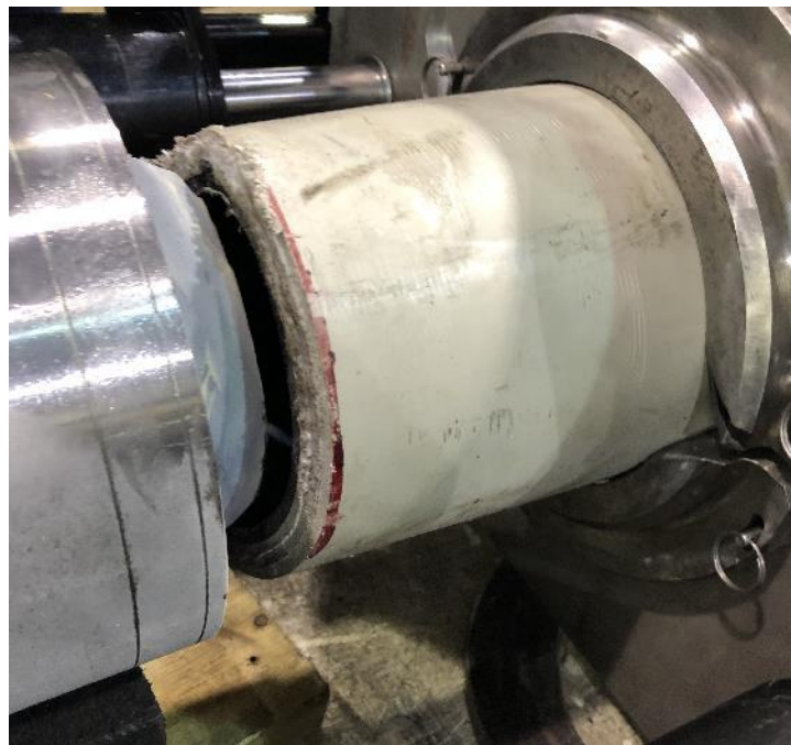
Figure 31: Pipe Clamp set closer for curved pipe insertion
