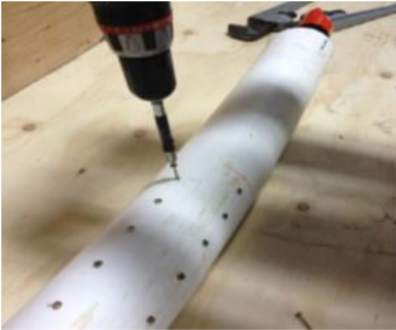
Figure 9: Securing Pipe with Screws
