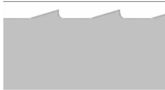
Figure 29: One-Way Teeth on the Pipe Clamp
