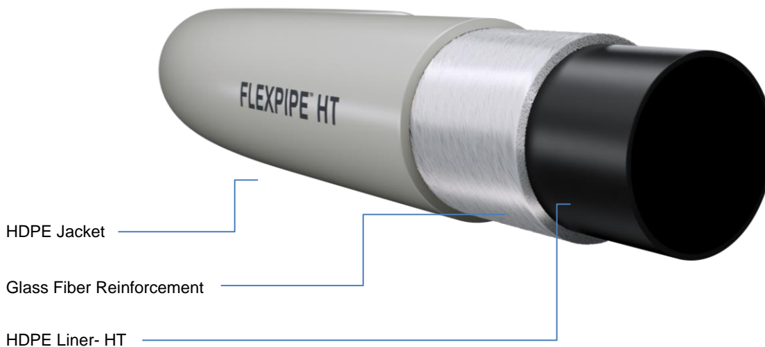
Figure 2: Flexpipe HT Design
